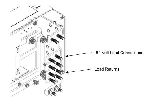
Figure 2.8-1 Connections to Circuit Breakers
